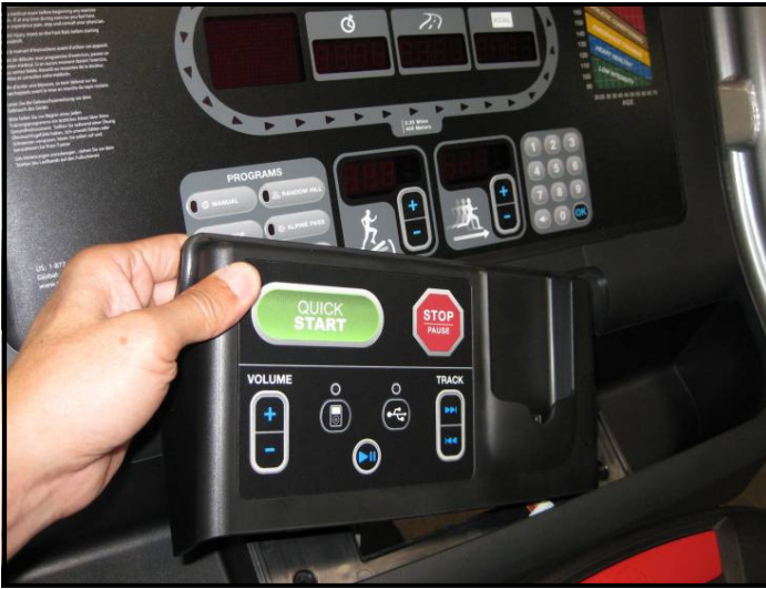
Step 9. Install the new iPod® center console.
